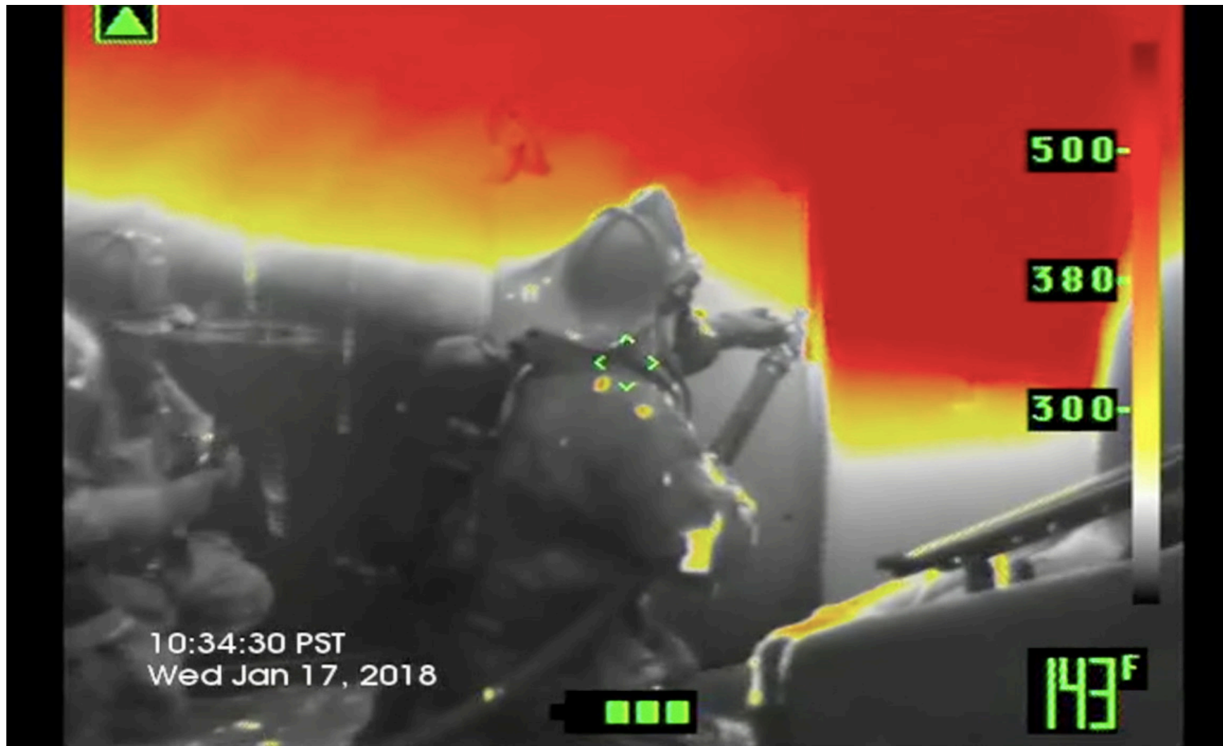
Image 4.7 This is the TIC image from a photo shown earlier in Chapter 3 (Image 3.5). The TIC is in the “low-sensitivity mode” looking toward the approach span from the entry span. Nozzle Forward photo.
