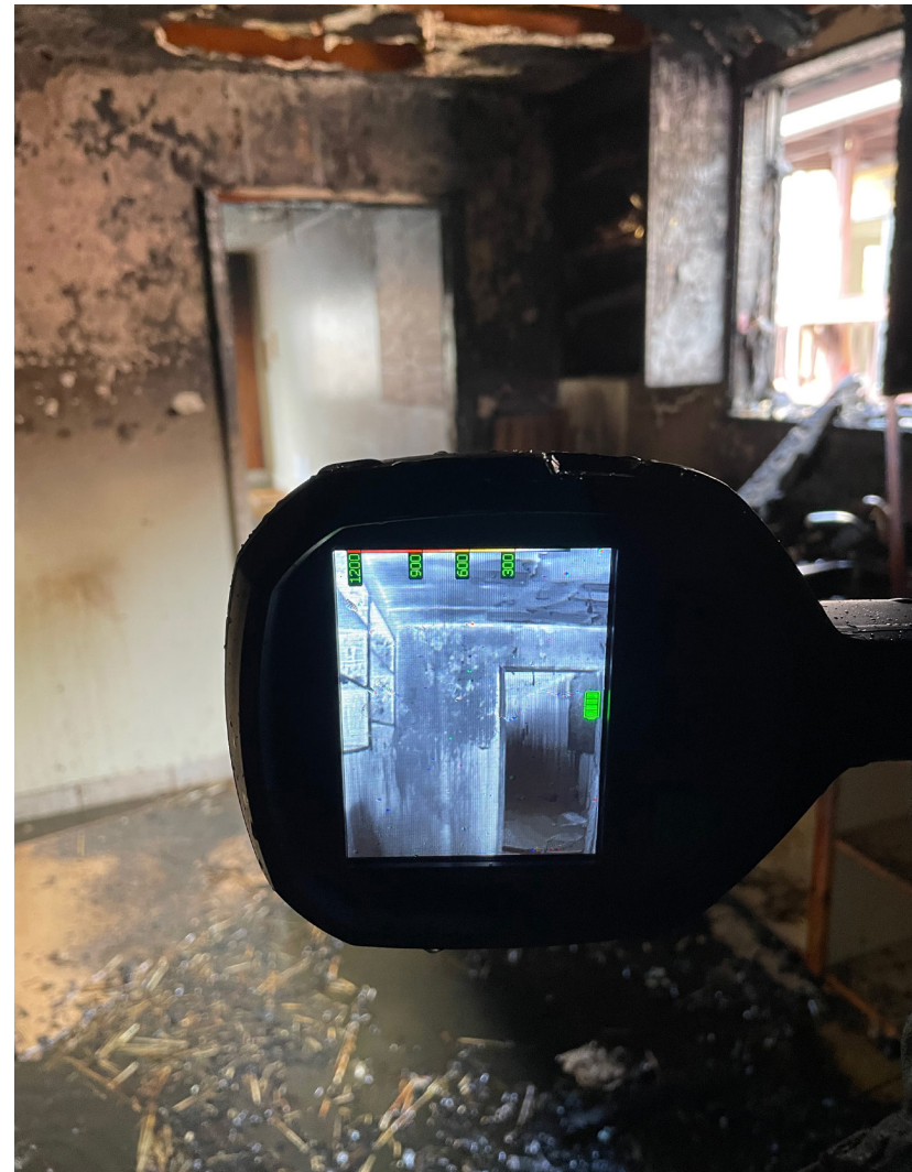
Image 4.6 A thermal imaging camera (TIC) in use after a fire. This image illustrates a depth disparity between vision and the image provided by the TIC. Jordan C. Legan photo.
